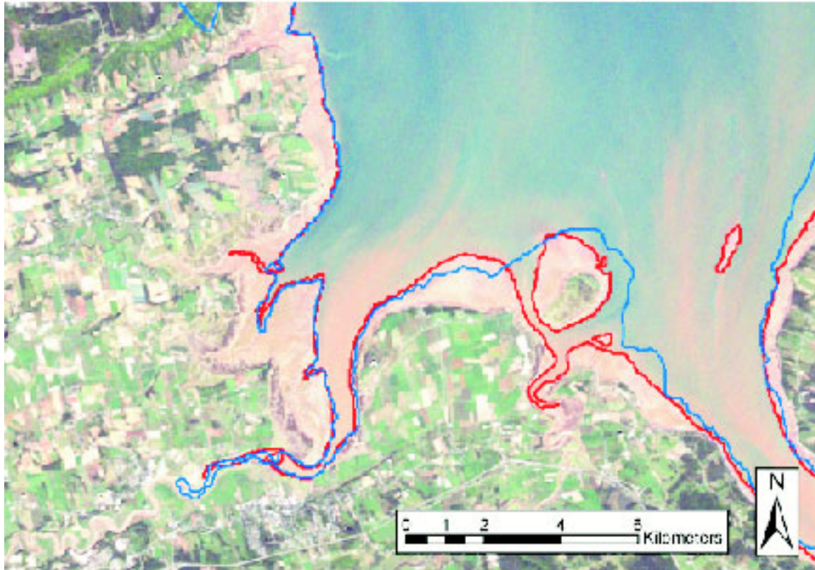
Figure 7: True colour Landsat-7 image of the Wolfville vicinity at 14:54:13 (GMT) on 13 Sept. 1999. The green is vegetation and the sandy brown is exposed tidal flats. The red line is the instantaneous coastline extracted from one of the near infrared bands and the blue line is the coastline extracted from the tidal model. The analysis is reported in Milne (2003). Courtesy of Trevor Milne (AGRG).
