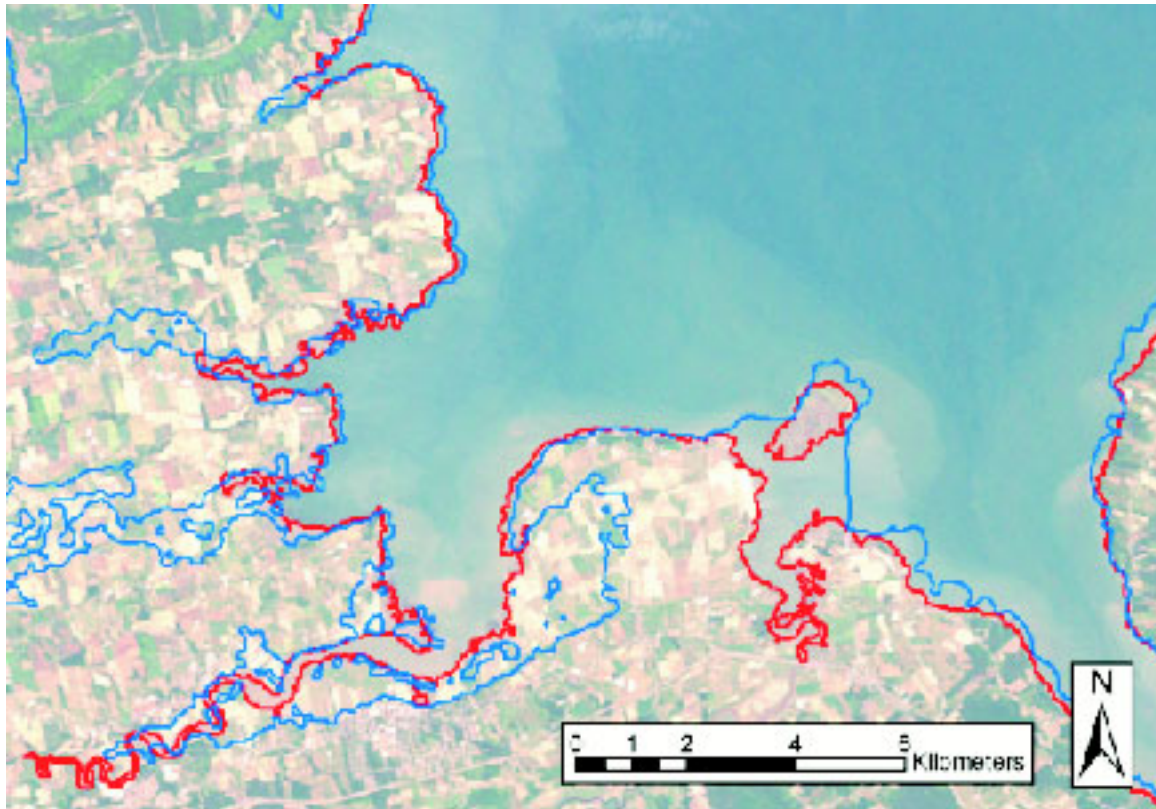
Figure 8: True colour Landsat-7 image of the Wolfville vicinity at 14:52:00 (GMT) on 13 July 2000. The red line is the instantaneous coastline extracted from one of the near infrared bands and the blue line is the coastline extracted from the tidal model. The analysis is reported in Milne (2003). Courtesy of Trevor Milne (AGRG).
