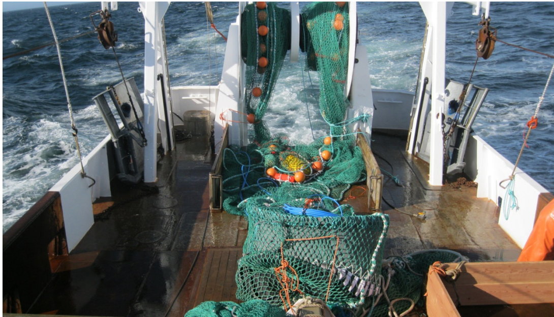
Figure 1. Sample net on the F/V Justice, November 2014. The hard container in the codend is the mounting for the video camera.
